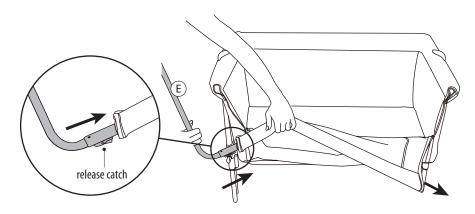
6a. Connect the upper tube to the main frame. A "click" will signal when secure.
