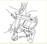
3. Press the button on the bumper bar and pull up in the meantime until take out from the stroller. press the button on the bumper bar and insert the bumper bar into the bumper bar interface, press the button to pop up, then bumper bar can be installed and fixed.
