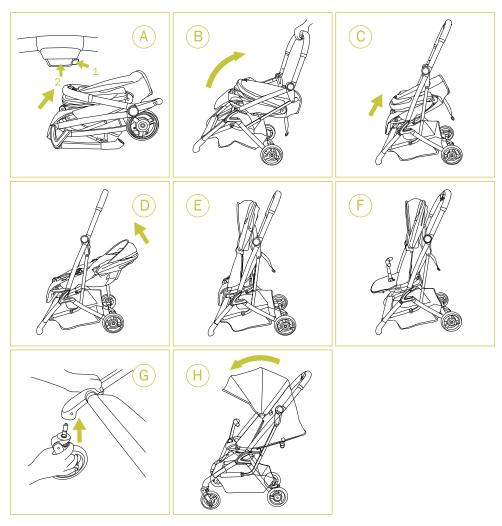
Unfold frame:see A,hold the hand grip by one hand,press button 1 and press button 2 in the meantiem, pull up the buggy until unfolded complete,see B. see C&D,lift the canopy back and up again,as shown in E.Then expand the bumper bar as shown in F to expand the frame. Install the front wheel: see G, insert the front wheel into the plastic hole of the front wheel until the click sound is heard, then install and fix the front wheel; see H, when the awning is opened, the platform is installed.
