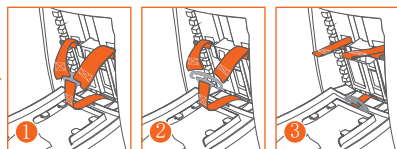
Step 3: Separate the shoulder belt with strap yoke: Put strap yoke into the rear cover and draw out the belt forward.
