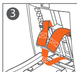
Step 3: Separate the shoulder belt with strap yoke: Put strap yoke into the rear cover and draw out the belt forward.
